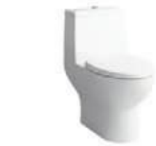
SAVOY H823947 One-piece floorstanding WC, siphonic action, Silent flush/rimless', Dual-Flush, including seat and cover, removable, with lowering system
