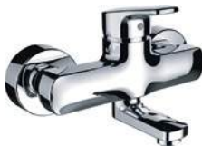
HF500921100600 Wall-mounted basin mixer, fittings distance 134–166 mm, projection 117 mm, swivel spout, with fittings, chrome
