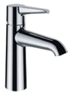
HF901702...000 Basin mixer, projection 110 mm, fixed spout, Eco+ function, without pop-up waste
