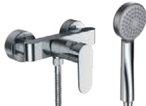
H3315170041311 Shower mixer, fittings distance 134–166 mm, with fittings, with synthetic flexible hose 1600 mm, with handspray Stella 80 1F, chrome
