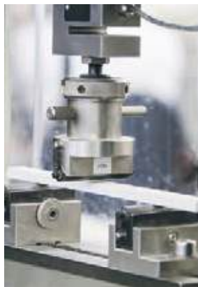
SAPHIRKERAMIK HAS A TWO TO THREE TIMES HIGHER BENDING RESISTANCE THAN TRADITIONAL CERAMICS
